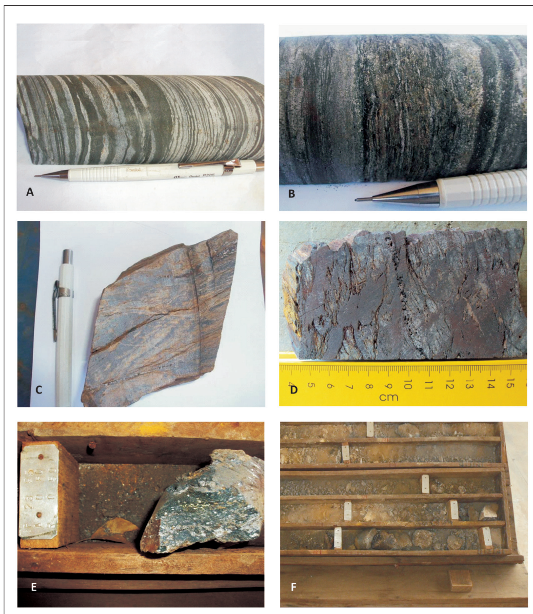
Figure 5 Banded iron formations (itabirites) drill-cores exhibiting some accounted geological features. A. Unweathered non-porous martitic itabirite (fresh rock); B. Slightly weathered amphibolitic itabirite; C. Moderately weathered hematitic itabirite; D. porous weathered hematitic itabirite; E. highly weathered magnetitic itabirite; F. friable highly weathered magnetitic itabirite.
